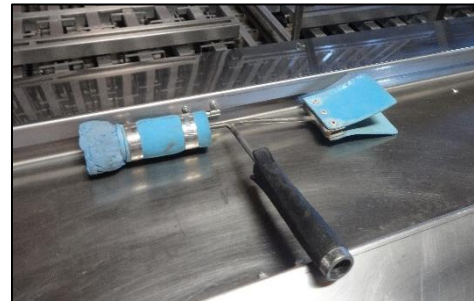
Product contact tools should be made of cleanable material and stored in appropriate locations to prevent contamination when not in use
