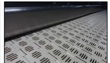
Guides that overlap conveyors
