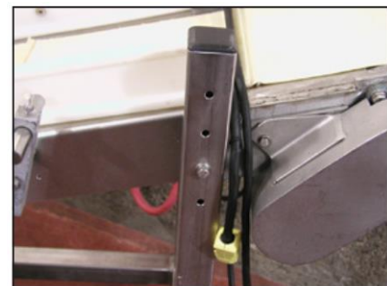
Seal holes in hollow frames and supports where moisture and Listeria can reside or replace with solid supports.
