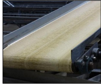
Old, cracked conveyor belts cannot be cleaned effectively and should be replaced.
